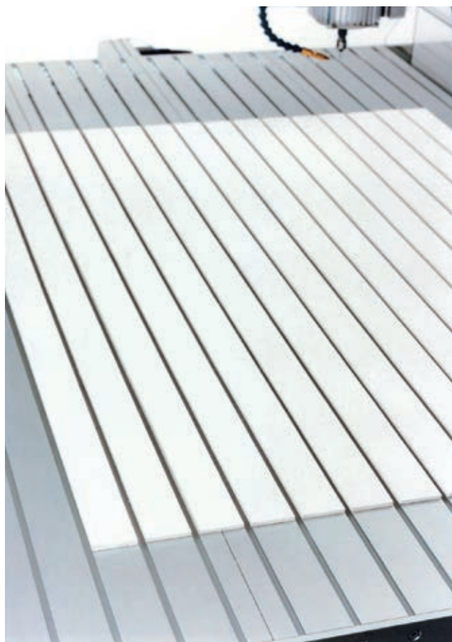
Trimmed polystyrene surface on the working table, the T-slots remain accessible here.
