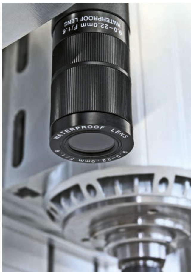
The CCD camera system captures register marks on the workpiece or the edges of the workpiece itself.
