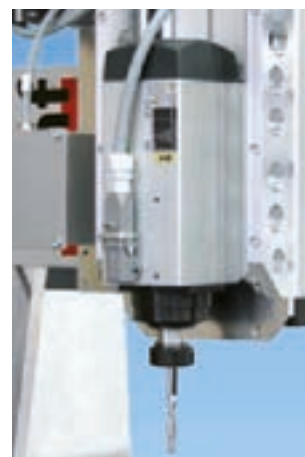
Power pack: SPC 6000 with 6 kW nominal power.
