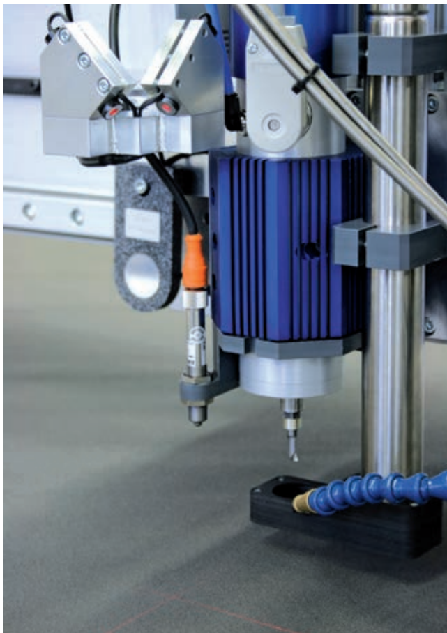
The line laser unit (top left) projects lines onto the machine table – using them, you can align your workpieces easily.
