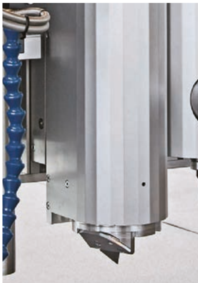
The universal head is suitable for many applications – here it is equipped with a V-cut knife for 45 degrees diagonal cutting.
