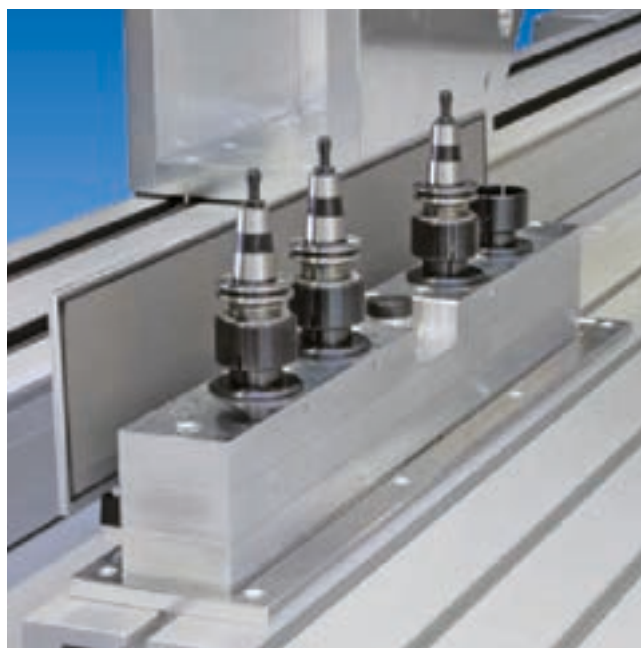
Cone change station WK 19: During the tool change process, the station automatically moves to the top, during the machining process it is protected by the lid from chips and oil mist.
