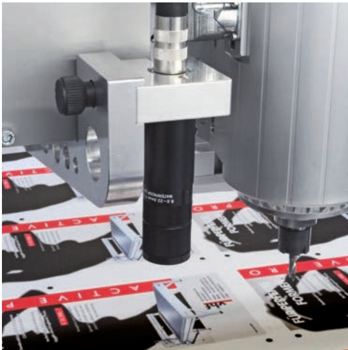
Cenon CCD captures the printed register marks and uses them for calculating the required rotation and scaling of the output paths.
