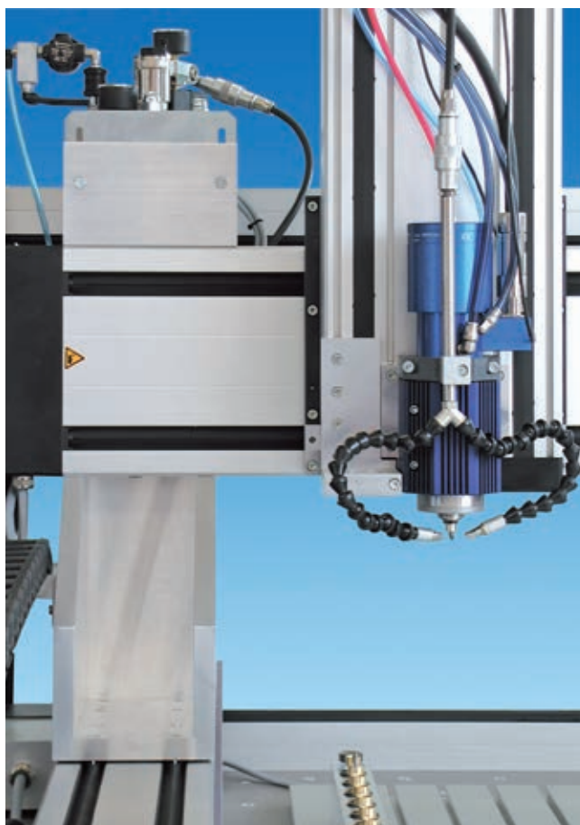
Minimum quantity lubrication with two flexible spray nozzles; top left: liquid tank with controls and instruments.
