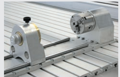
Rotary axis type S with three-jaw chuck (right) and tailstock unit with centre sleeve (left).
