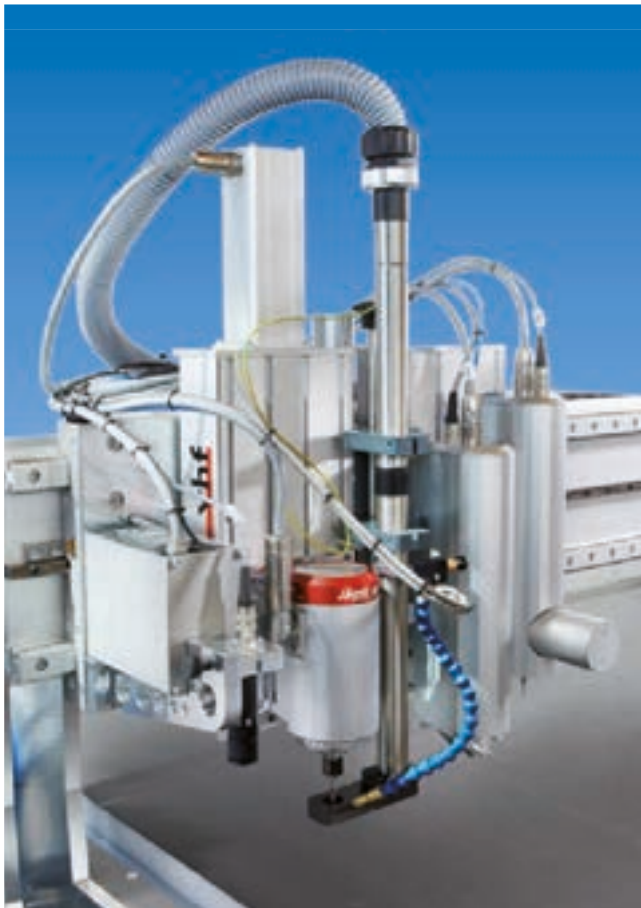
A multi unit (mounted right of the suction unit) is recommended when you often have to use different machining techniques.
