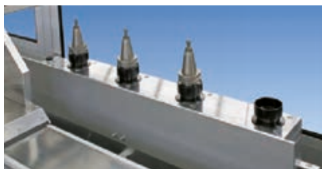
Cone change station SK 30: The station is located in a separate area outside the actual machine table.
