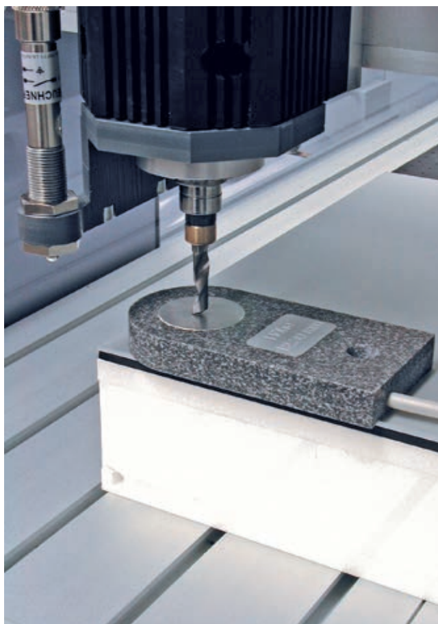
Adjustment of the z origin of a workpiece within seconds with the mobile measuring plate.
