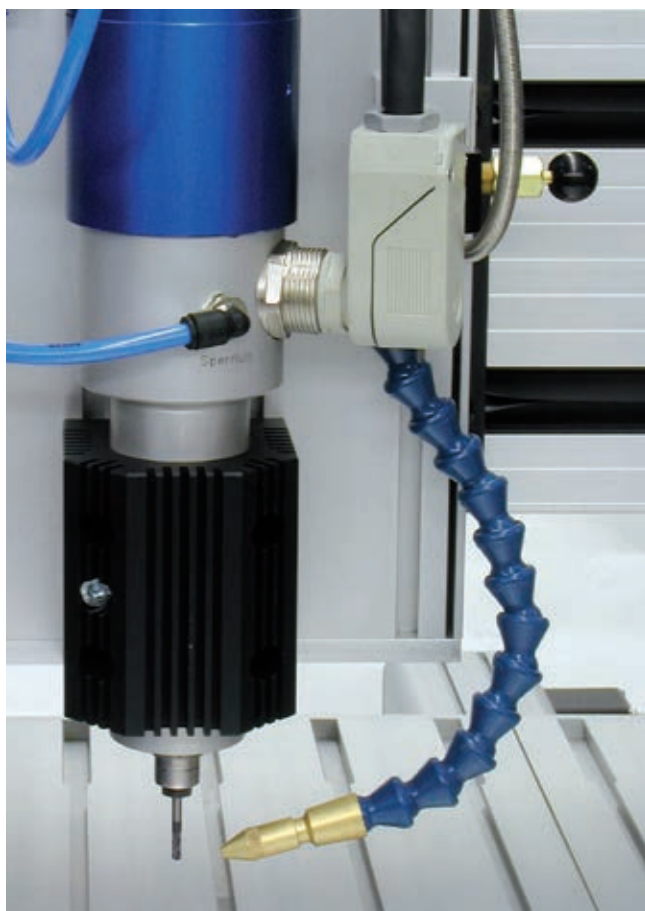
Manually controlled cooling/spraying unit (right of the high frequency spindle).
