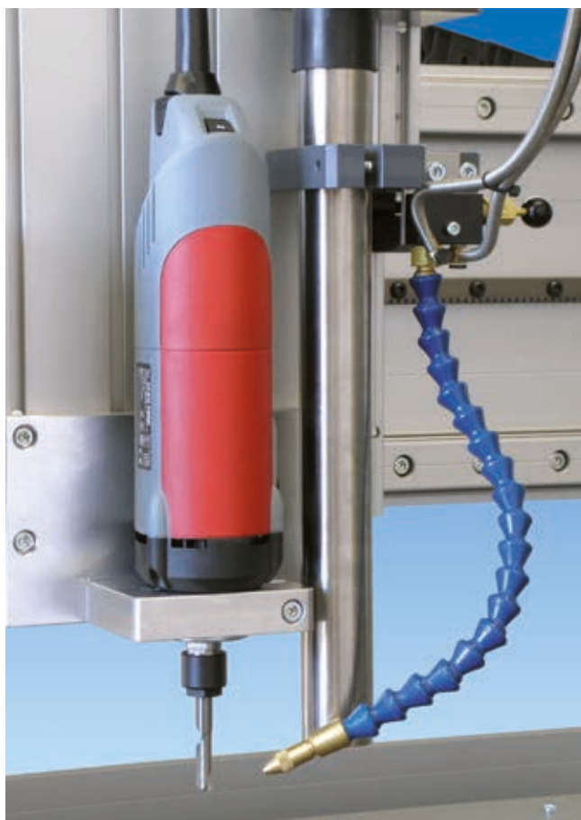
Standard spindle – a good-value alternative for tasks which do not demand high precision.
