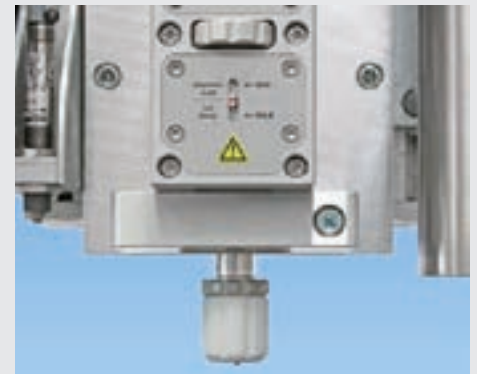
The lance emerges a little bit from the distance bush; the thumb wheel is used for setting the pressing force.
