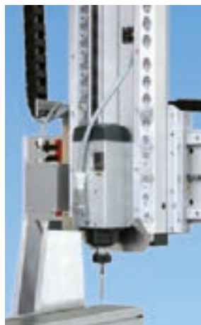
Detail view of the additionally reinforced z axis with a lift of 700 mm (here a rotary current spindle SPC 6000 is mounted).
